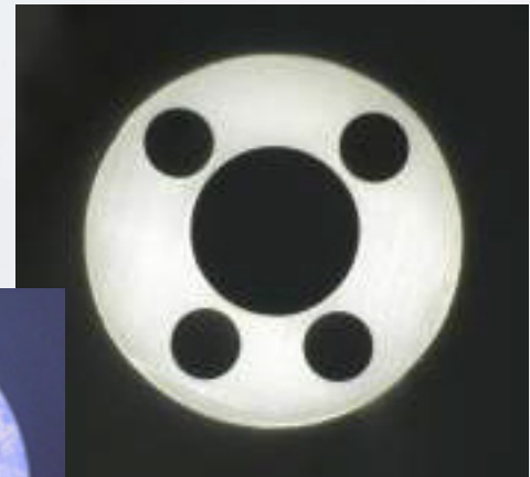
Cross section of multi lumen tube
