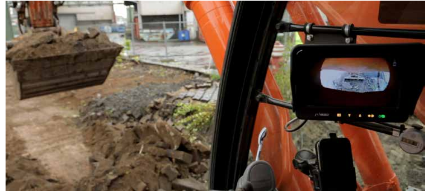
Load monitoring with the MC7180 heavy-duty camera.
