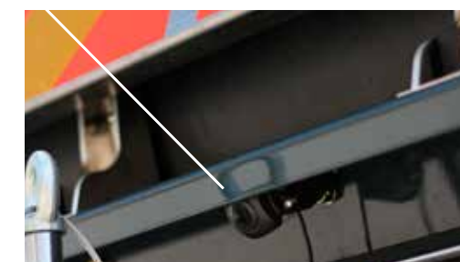
Putzmeister concrete pump truck with front camera, ultrasound and radar sensor, side monitoring and rear space monitoring.
