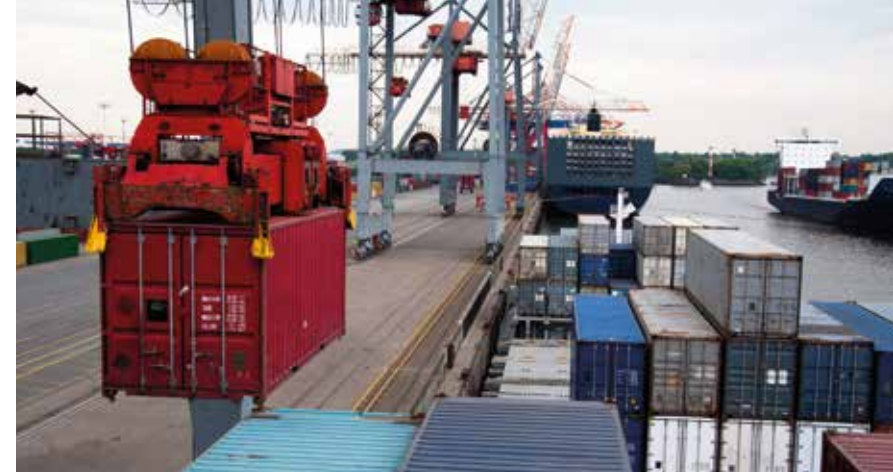
Rail-bound mobile harbour crane handling containers.
